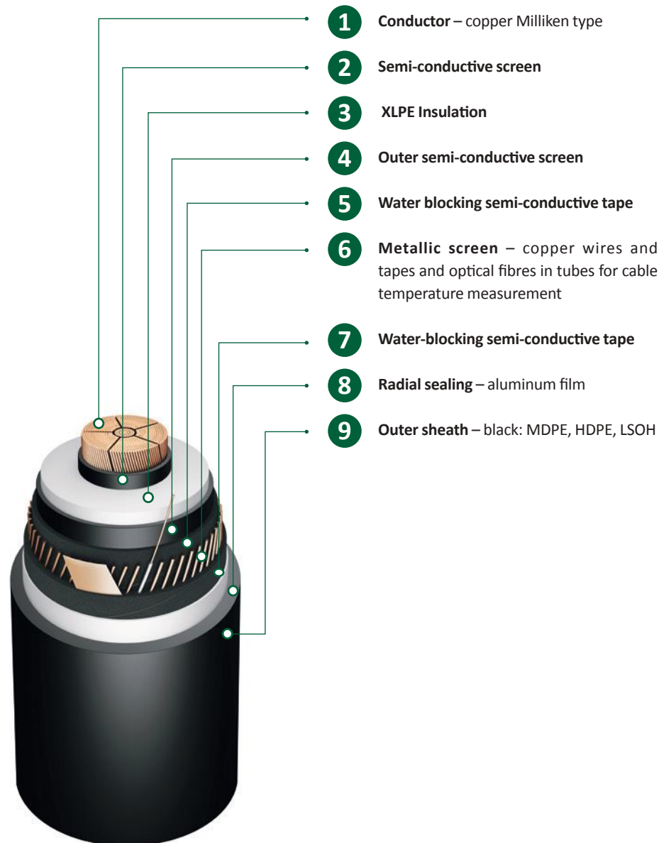
Image 18. N2XS(FL)2Y 1x2500 400kV description:
